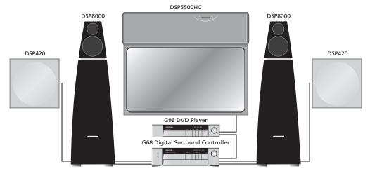
The G68 Digital Surround Controller can be used with Meridian digital loudspeakers, such as DSP8000s and a DSP5500HC centre speaker, to provide audiophile quality sound. A further two or four speakers, such as DSP420 Digital Loudspeakers, can be added as side or rear loudspeakers to give excellent multichannel reproduction from music and movie sources.
